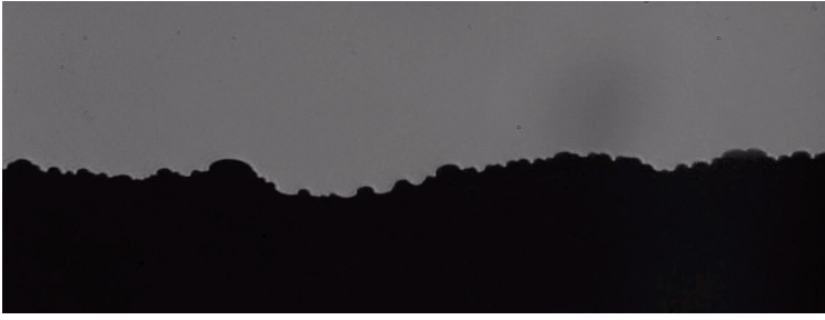
Figure 6.1: Left: Snapshot of a contact-line at depinning, courtesy E. Rolley [movie]. Right: Velocity of a pinned interface as a function of the applied force. Zero force: equilibrium. f = f_c : depinning.
